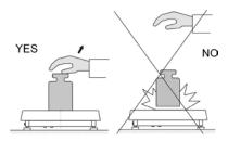
Loads should be placed centrally on the pan (errors caused by eccentric weighing are outlined by standard PN-EN 45501 ch. 3.5 and 3.6.2):
