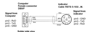
Scale - computer cable diagram for metal housing
