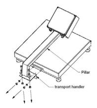
Turn the pillar and mount it to the platform. The surplus cable place inside the pillar.
