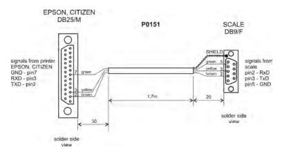
Scale – printer cable diagram for plastic casing
