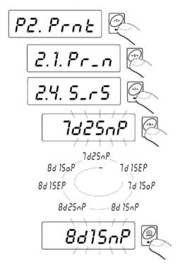
7d2SnP - 7 data bits; 2 stop bits, no parity control
