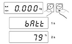
After displaying the level of batteries (in per cents) the program returns to weighing.
