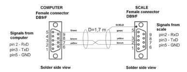
Scale - computer cable diagram for plastic casing
