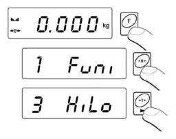
• The program enters the window of setting the lower threshold of weighing (**Min**):
