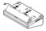
Remove discharged and then insert new batteries into the chamber, according to given polarity (+/-):
