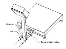
Pick up the pan and remove the transport protection.
